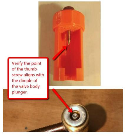
When the system is off, the refrigerant pressures on both sides of the EEV plunger will be close to the same. The plunger travel is less than  $\frac{1}{2}$ " and does not require a lot of force to seat it. Be careful not to not apply excessive torque or damage to the tool may occur.
